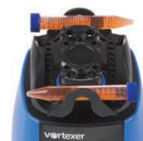
15 mL conical tubes x 2 (horizontally mounted)
